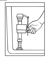
Turn on water supply. Adjust water to desired level by squeezing water level adjustment clip and moving FLOAT CUP up or down along stainless steel link
