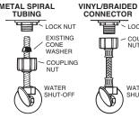
Use existing spiral cone washer. Fluidmaster cone washer may not seal completely on spiral type supply
