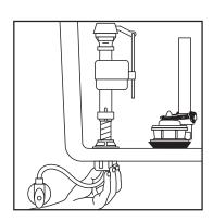
With correct washers in place (see Step 9a), tighten COUPLING NUT 1/4 turn beyond hand tight. DO NOT OVERTIGHTEN.
